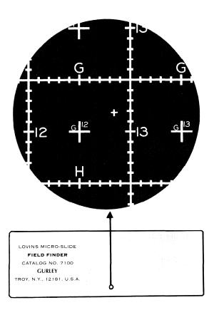
The Lovins Micro-Slide Field Finder is a simple precision device for the microscopist to relocate fields of interest in a slide-mounted specimen.
